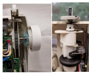
Avoid putting your spool of thread to the right of your machine where it can get wrapped around the hand wheel. When winding a bobbin take care it is not winding around the spindle instead of the bobbin.
